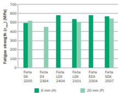
Fig 9. Fatigue strength, 50% probability of failure at 2 million cycles, tested with R = 0.1 , F = 20 Hz.
