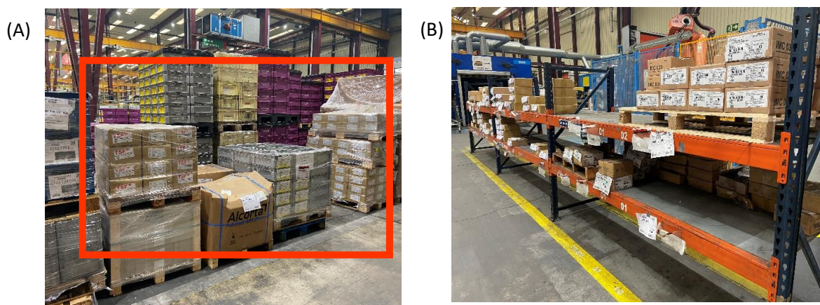
Figure 13 – (A) Child-part components in the supermarket; (B) Child-part rack
