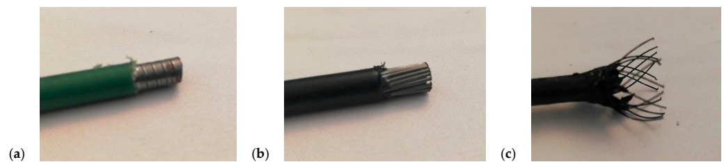
Figure 6. Spiral types: laminated spiral without inner tube (a), push-pull spiral (b), and braided spiral (c).
