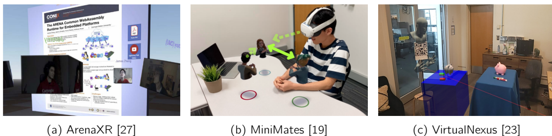
Figure 2.3: Extended reality telepresence examples: In (a), users are represented as video-cube avatars while interacting in a VR scene. In (b), the AR user sees others represented as miniature avatars, which are projected onto his real-world perspective. Combining both AR and VR, (c) demonstrates MR telepresence, allowing a VR user, projected as an avatar, to experience the same physical location as an AR user.
