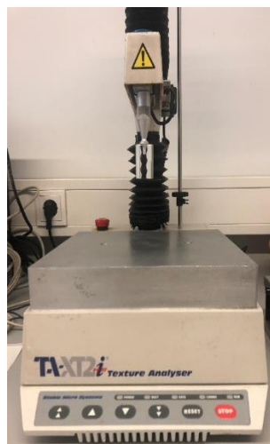
Figure 8. Texture analyser TA-XT2i, Stable Micro Systems (United Kingdom).
