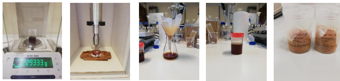
Figure 2. Scheme of extraction process of L. barbarum berries
