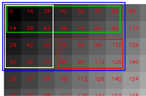
Figure 1. Example of any rectangle in the image, in red. The sum of the values of its pixels is equal to the sum of those in the blue rectangle minus those in the green rectangle minus those in the white rectangle and replacing once those in the overlap between the green and the white, since they were subtracted twice.
