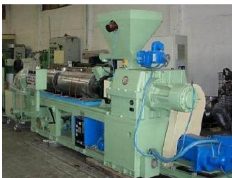
Figure 11. Extrusion machine with PM motor
