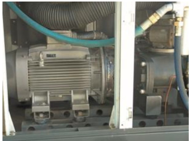
Figure 6. Compressor with PM motor
