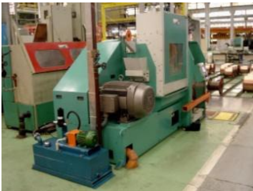
Figure 8. Wire drawing machine with PM motor
