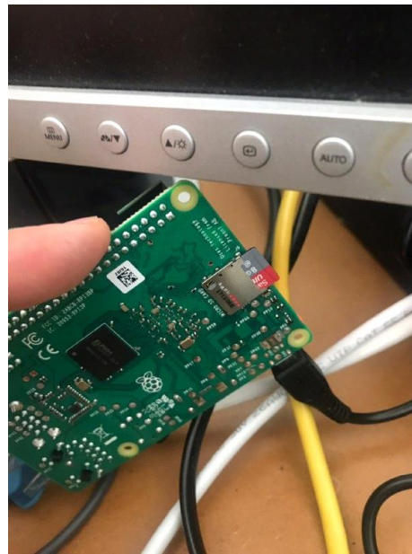
Figure 60 Port for micro sd card in Raspberry PI
