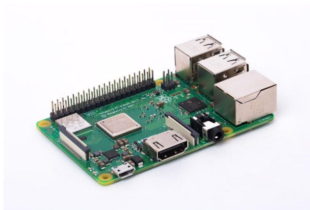
Figure 6 Raspberry PI 3B
