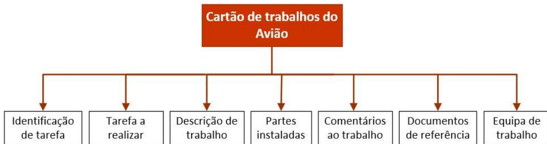
Figura 42 - Diagrama Aircraft Work Card
