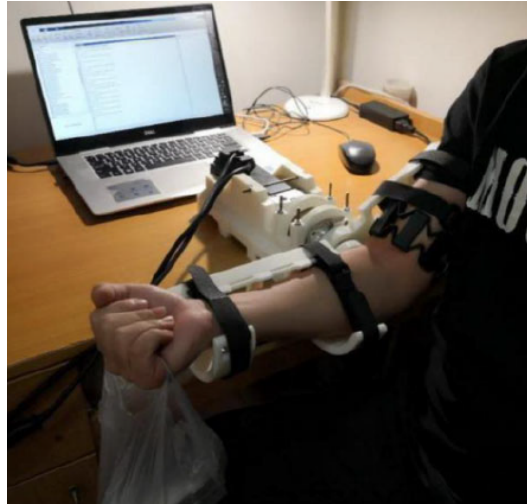
Figure 3.4: Structure based in 3D printing for an exoskeleton actuated system [71].
