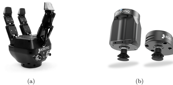
Figure 2.3: Anthropomimetic plus a non-biomimetic and non anthropomimetic end-effectors (a) A three finger gripper (anthropomimetic) [45]. (b) A vacuum gripper (non-biomimetic and non-anthropomimetic). [47].
