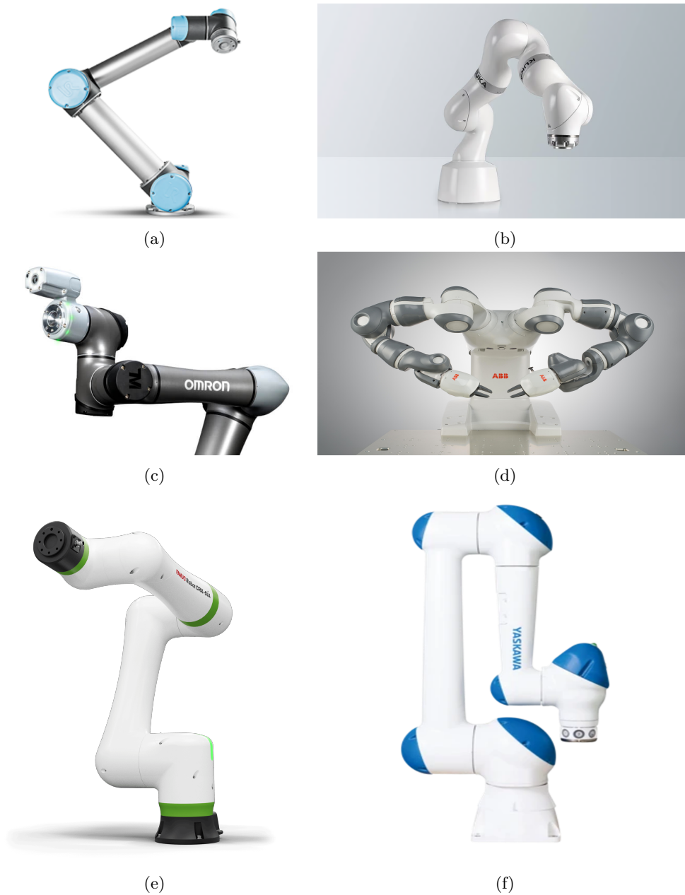
Figure 2.1: Robotic manipulator models: (a) UR5 model [26]; (b) KUKA LBR Med model [27]; (c) TM5-700 model [28]; (d) YUMI IRB 14000 model [29]; (e) FANUC CRX model [30]; (f) YASKAWA HC10DTP model [31].
