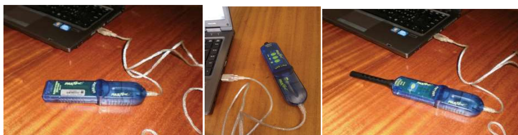
Figure 1 - Photographs of three sensors used to characterize the School's indoor environment: Humidity and temperature sensor (Pasco PS - 2124); light sensor (Pasco PS - 2106A) and carbon dioxide sensor (Pasco PS - 2110)
