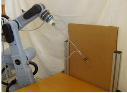
Fig. 2. Steel rod impact against a rigid surface
