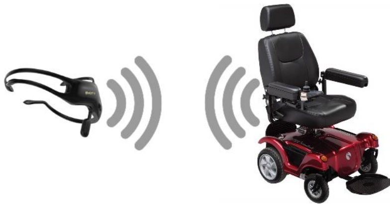
Figure 21 - Direct connection between BCI headset and mobility aid
