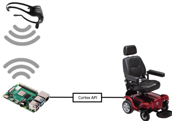
Figure 22 - Indirect connection between BCI headset and mobility aid
