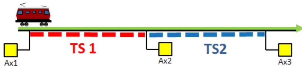
Figure 2.7: Axle Counters for train detection. (Palumbo, 2013)
