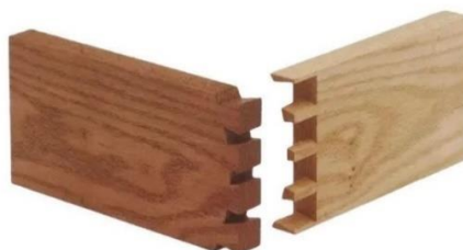
Figura 21 - Junta de Cauda de Andorinha Passante Curvada “Curved Through Dovetail”. Home-Douglas et al. 1993. Handbook of Joinery (Art of Woodworking) .
