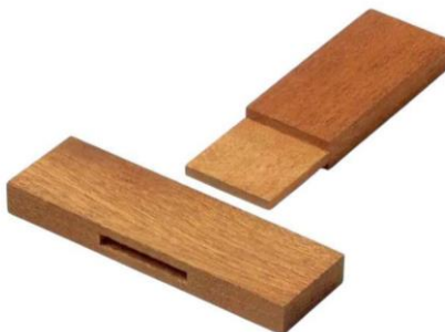
Figura 22 - Junta de Furo e Espiga Passante “Through Mortise and Tenon” Jackson, A., Day, D. 1995. Good Wood Joints .
