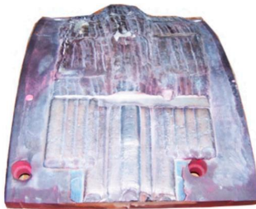
Figure 18 - Final result of a component produced by 3DPMD[69]
