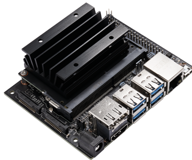
Figure 2.11: NVIDIA Jetson Nano for AI [33]
