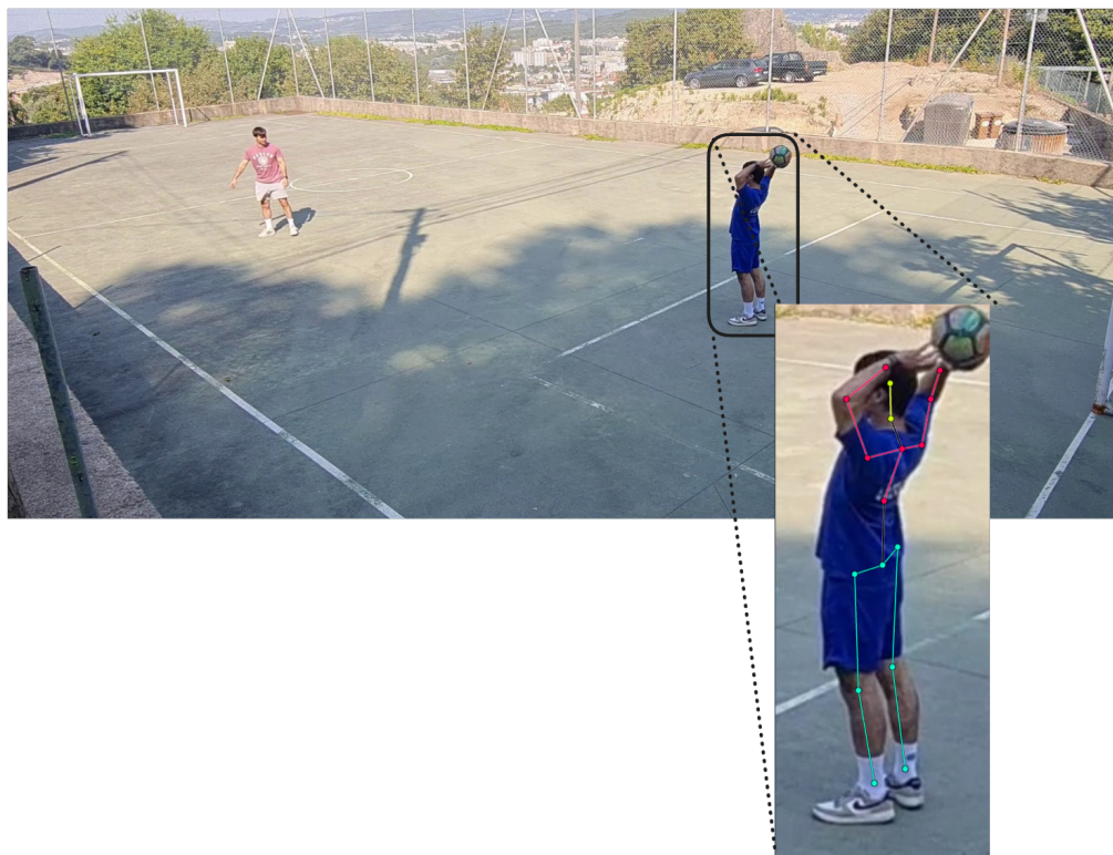
Figure 3.17: Player detected committing a handball violation pose estimation identifies hand contact with the ball
