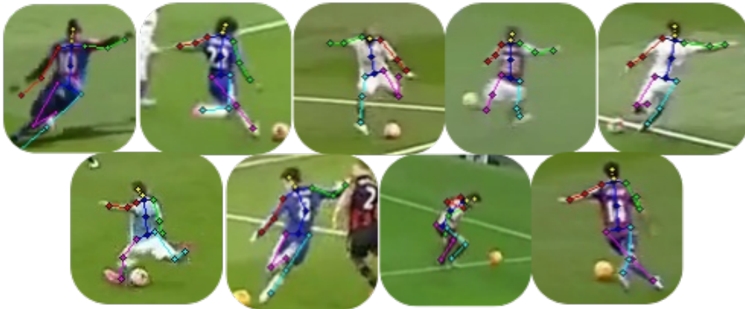
Figure 3.14: 3D Shot Posture Dataset showing various player shooting poses with keypoint annotations including neck, center body, center of shoulder, and center of hips
