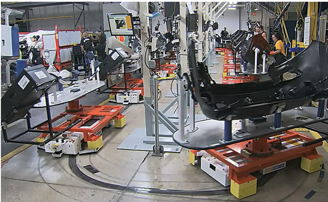
Figure 13 - Automated guided cars in assembly line application [55]
