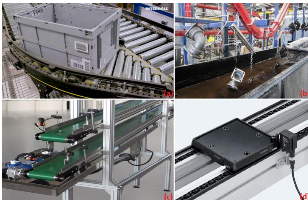
Figure 12 - a) Roller conveyor [48]; b) Overhead conveyor [49]; c) Belt conveyor [50]; d) Chain conveyor [51];
