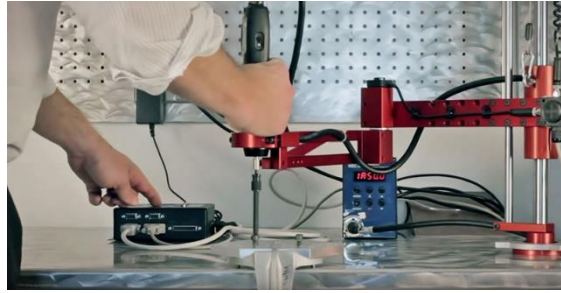
Figure 11 - Positioning torque arm with an electric screwdriver [43]
