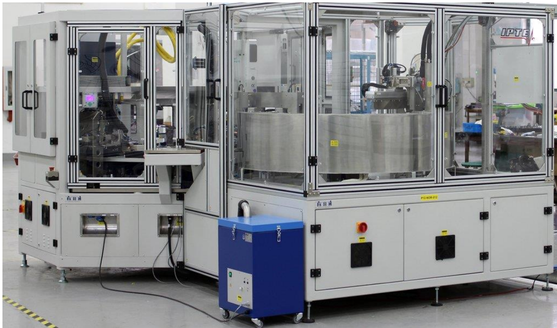
Figure 15 - Machine example with a lower welded steel frame and an upper frame made with aluminum profile
