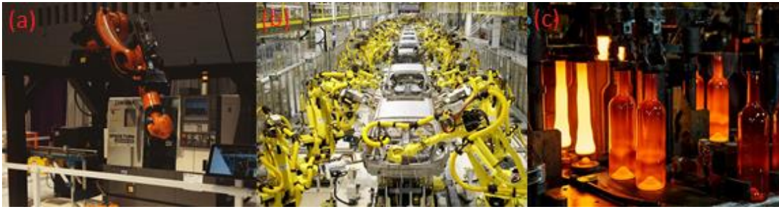
Figure 8 - Examples of: a) Programmable automation [29]; b) Flexible automation [30]; c) Fixed automation [31];
