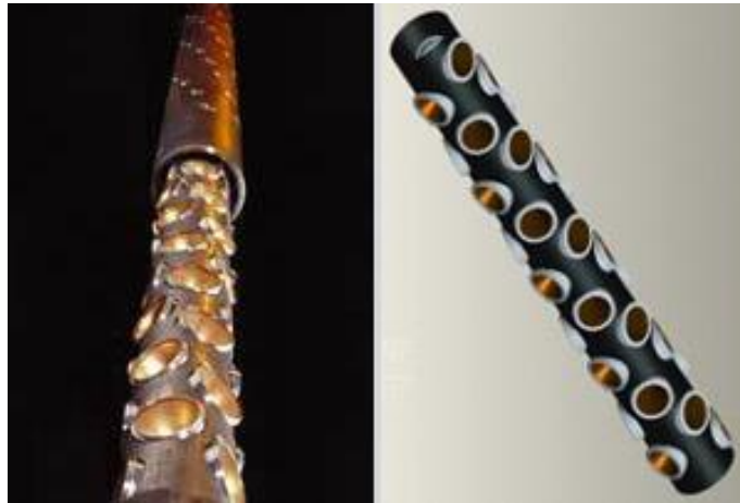
Figura 65. Perfurador, (adaptado de: “Perforating Gun”,LANDSEA products, lsea.com).
