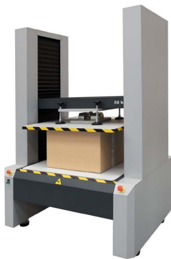
Figura 30 – Ensaio BCT, norma ASTM D642 [43]
