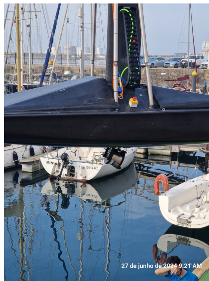
Figure 5.13: M3 Kongsberg sonar on the USV PORTUS.
