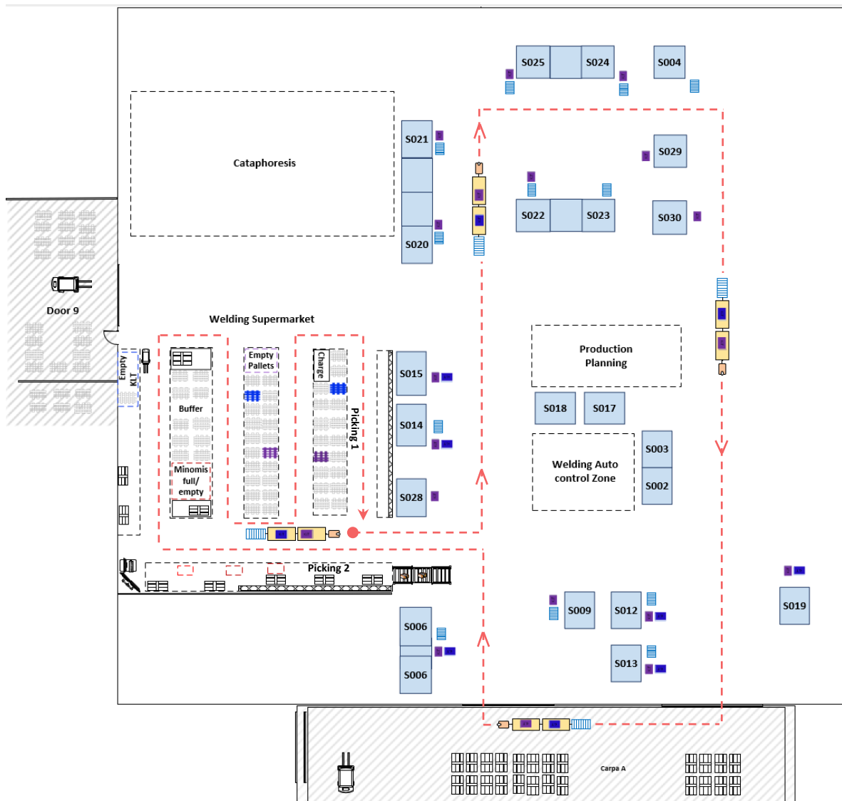
Figure 49 – Mapping 1): parts supply flow from the supermarket to the cells border of line. Source: Own Elaboration
