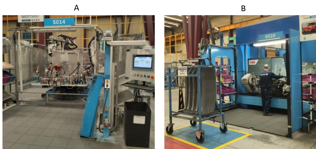
Figure 24 - Resistance and MAG welding cells
