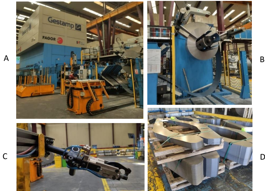
Figure 22 – Stamping process (Transfer line)
