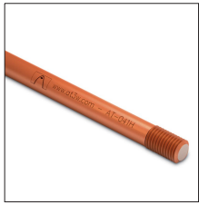
AT-041H \phi 5/8"x2m thrd 254 \mu Cu- bond earth rod
