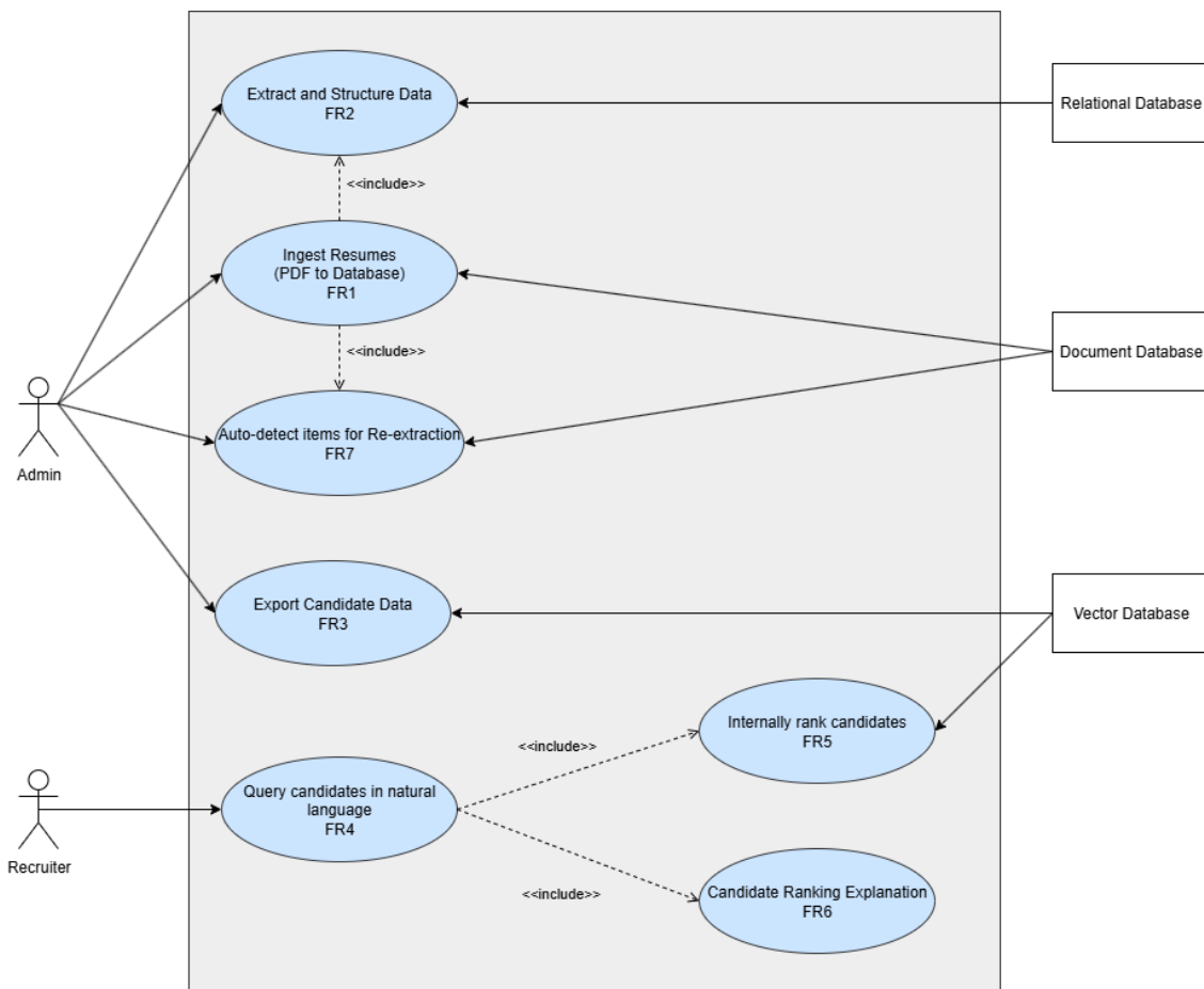
Figure 4.1: Use-Case Diagram for LLM-Powered Resume Matcher
