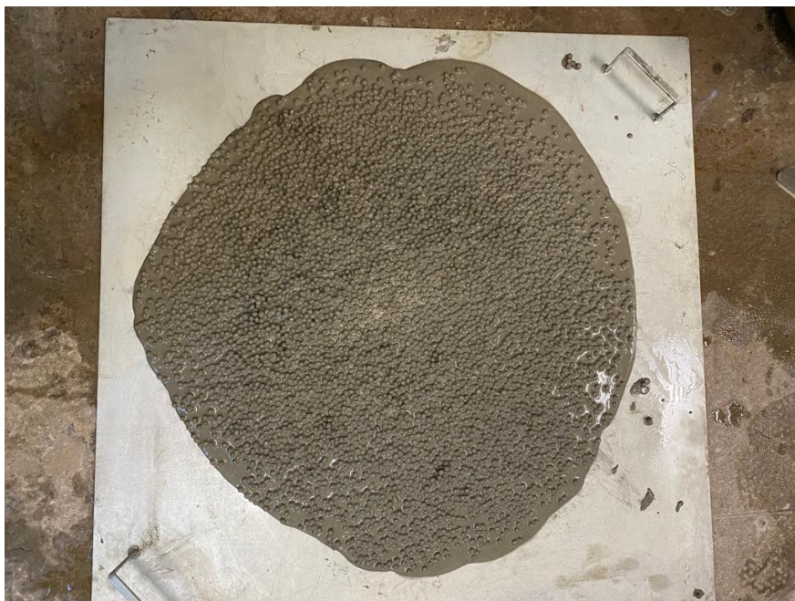
Figura 4.3 – Foto slump flow TEPS1.
