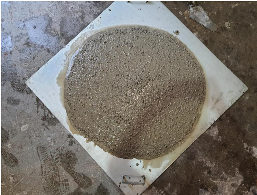
Figura 4.1 – Foto slump flow TREF.
