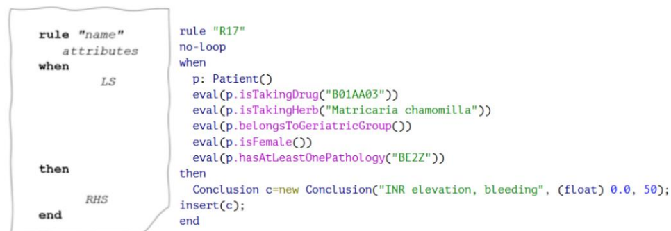
Figure 8 - Standard structure (left) and example (right) of a When-Then rule.
