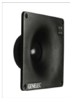
The tweeter driver is mounted in a DCW to match the dispersion characteristics to that of the bass driver. The DCW may be rotated for horizontal or vertical mounting.
