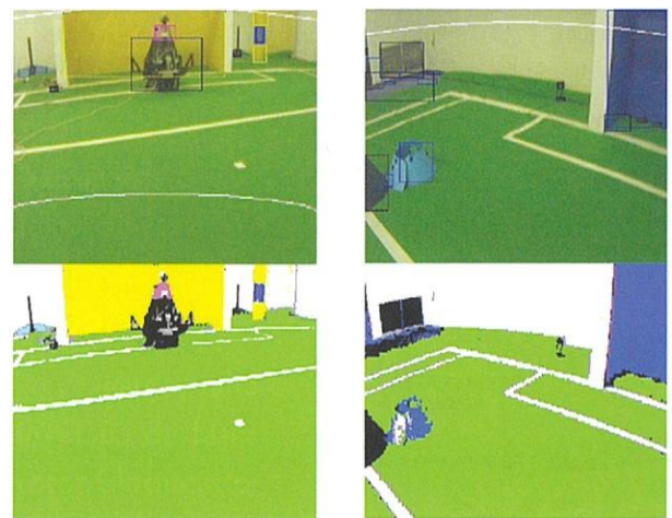
Figure 5 · Example of robot vision blob algorithm and edge finding algorithm.
