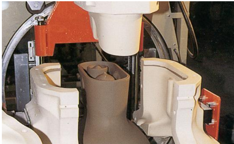
Figure 8 – Demoulding the workpiece from three portions of the mould [23]
