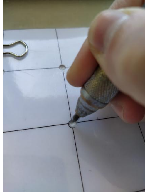
Figure 45 – Percussion pen provoking defects
