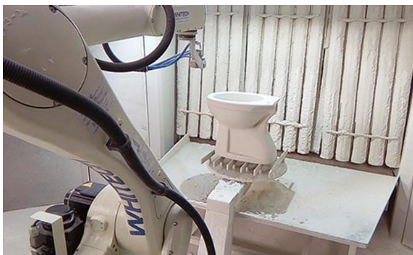
Figure 10 – Application of the glaze to the workpiece using a robotic arm [23]
