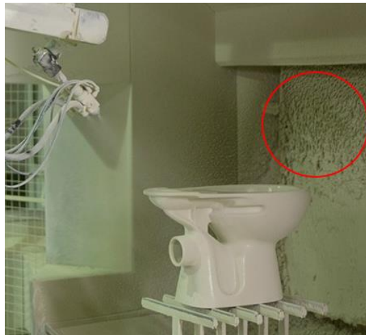
Figure 16 – Residual waters formed during the application of the glaze (adapted from [28])
