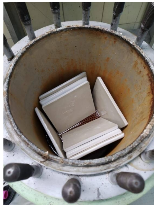
Figure 114 – Specimens in the autoclave
