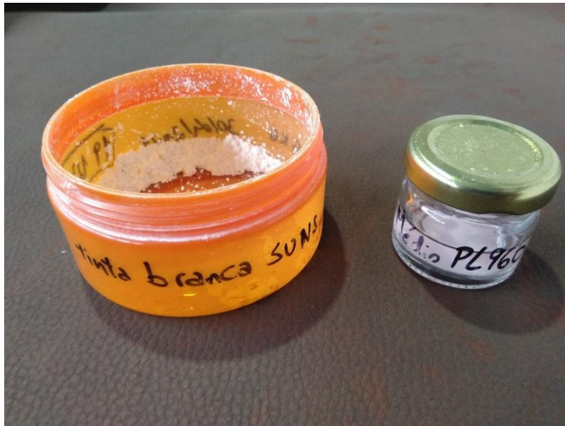
Figure 76 – White ink formed with diluted PL960
