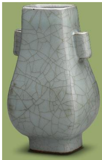
Figure 40 – Crazing in ceramic faience [84]
