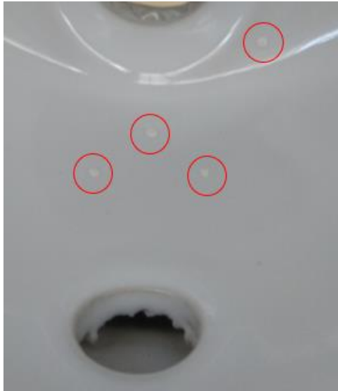
Figure 22 – Repaired defect - Pinholes
