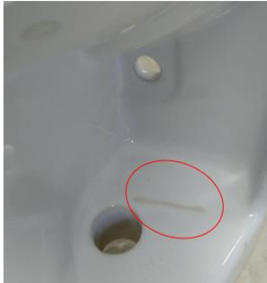
Figure 23 – Repaired defect - Crack
