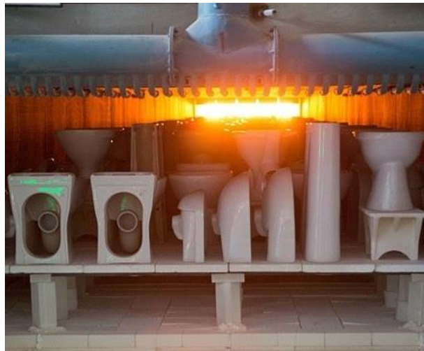
Figure 13 – Sanitary ware firing [28]
