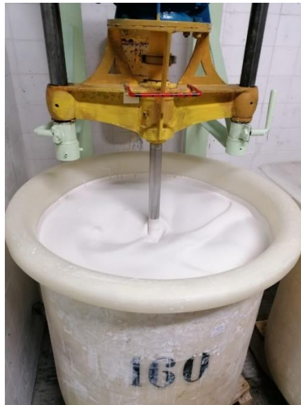
Figure 14 – Glaze in the mixing tank
