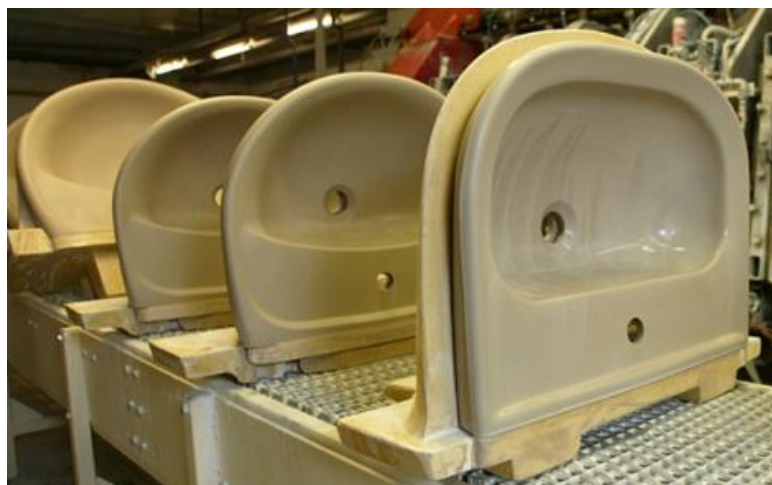
Figure 5 – Sanitary ware production (adapted from [11])
