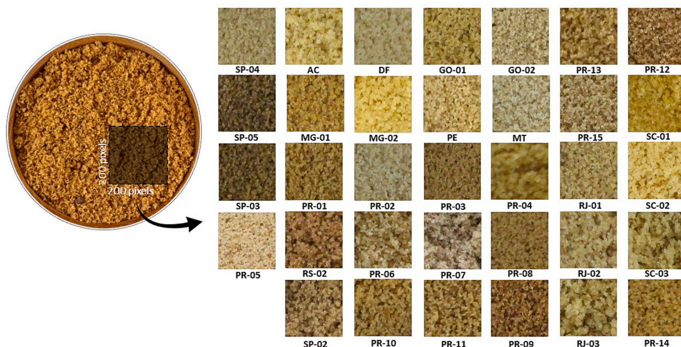
Fig. 2. On the right, ROIs (Region of Interest) of Brazilian brown sugar samples with their respective encoding. On the left, an illustration of the ROI with dimensions of 200 x 200 pixels obtained by cropping the original image.
