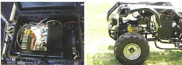
Figure 2. Robot main electronics and CPU box (left) and direction (right) details.
