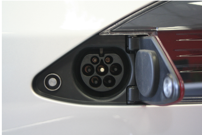
Figure 2.5: Tesla socket inlet modified for Mennekes plug [16]
