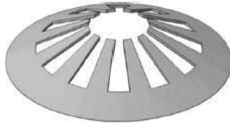
Figure 27 – Simple form of a diaphragm spring (Mashadi & Crolla, 2012)
