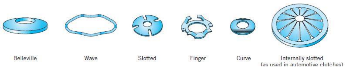
Figure 26 – Types of spring washers (Juvinall & Marshek, 2012)
