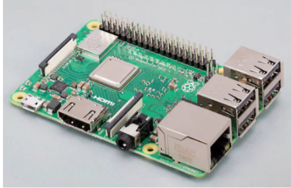
Figura 4.21: Raspberry Pi 3 modelo B+.
