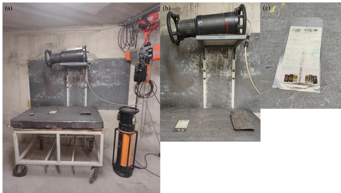
Figure 15 – Experimental radiographic inspection setup adopted throughout the inspection campaign: (a) general view of the X-ray inspection system; (b) portable X-ray source used during radiographic exposure; (c) positioning of the impacted specimen over the radiographic film prior to X-ray exposure.
