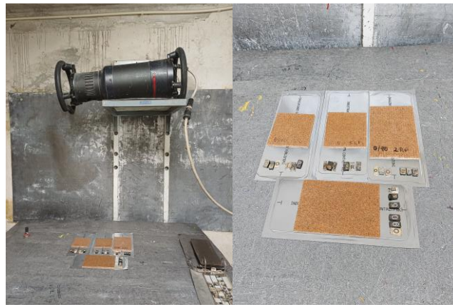
Figure 16 – Setup adopted for the radiographic inspection and specimen positioning prior to X-ray exposure.
