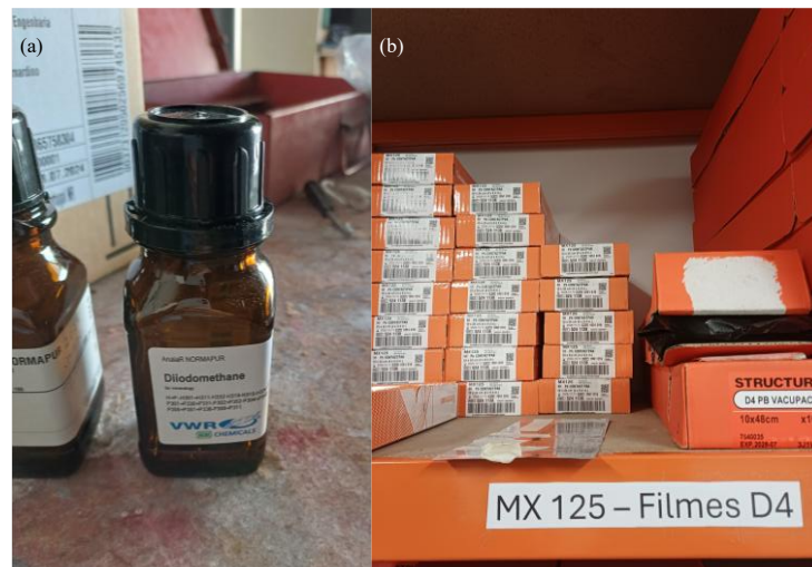
Figure 14 – Materials used during the radiographic inspection procedure: (a) diiodomethane contrast agent; (b) MX125 D4 industrial radiographic films.
