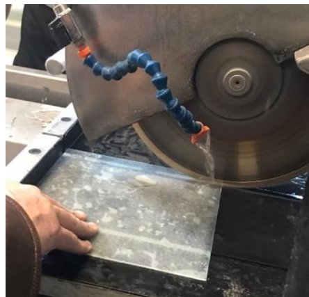
Figure 12 – Cutting process adopted for the preparation of the composite test specimens.
