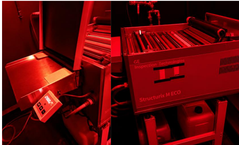
Figure 17 – Darkroom radiographic film processing equipment and processing workflow.
