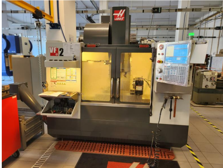
Figure 13 - CNC machining center HAAS VF-2 (HAAS Automation, Oxnard, CA, USA).
