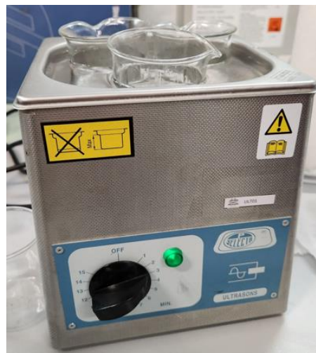
Figure 18 - Equipment used for ultrasonic cleaning of tools.
