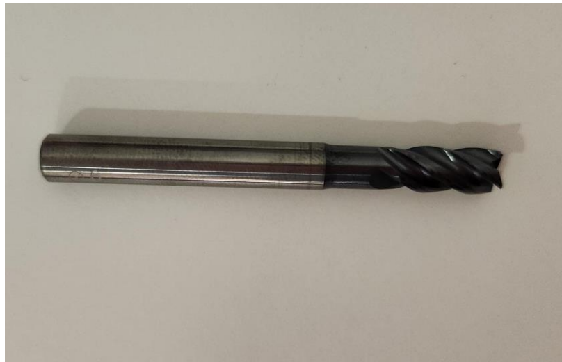
Figure 12 - Cutting tool coated with TiN/TiAlN multilayer coating.
