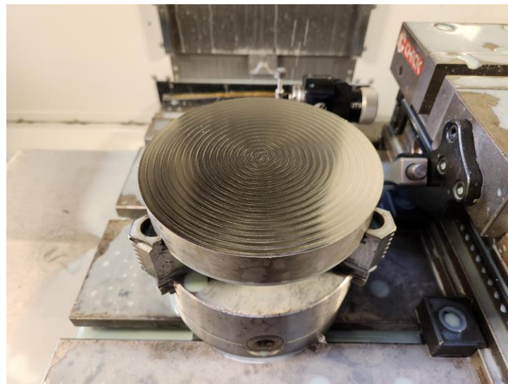
Figure 14 - Assembly of the Inconel 718 part to be machined.
