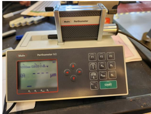
Figure 17 - Mahr Perthometer M2 profilometer
