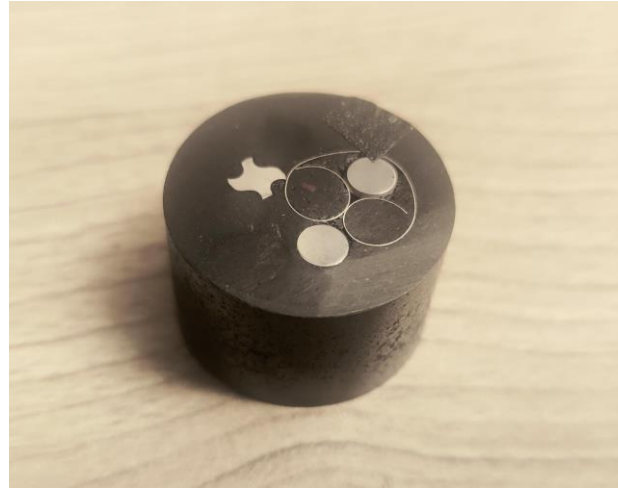
Figure 16 - Sample embedded in thermosetting resin.
