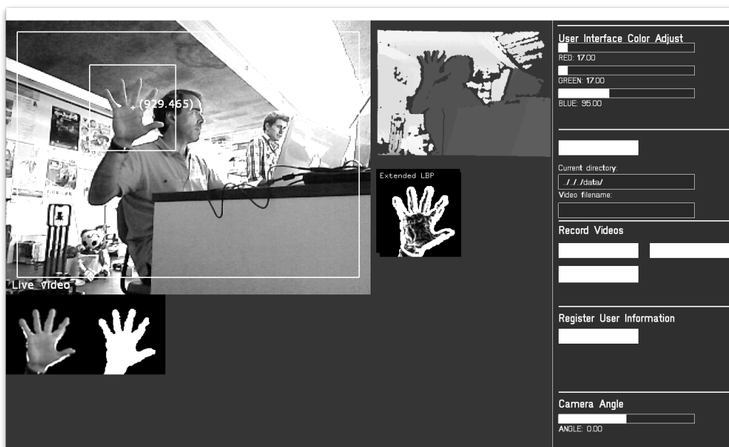
Figure 72. Local Binary Pattern operator feature extraction.
