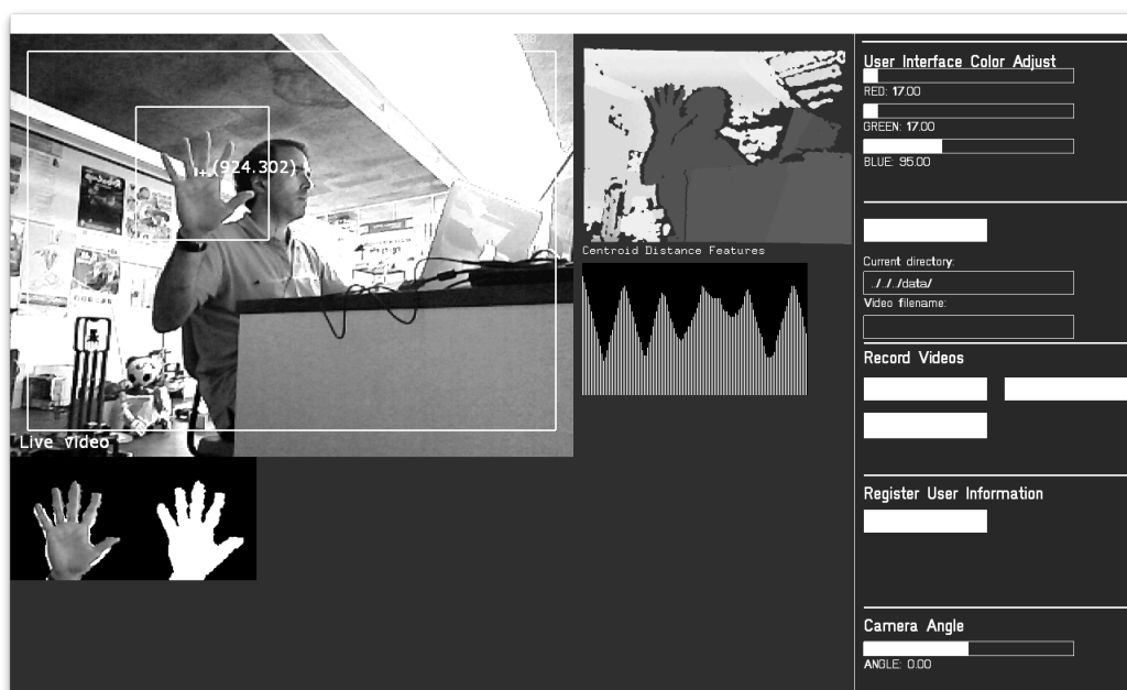
Figure 76. Centroid Distance operator feature extraction.
