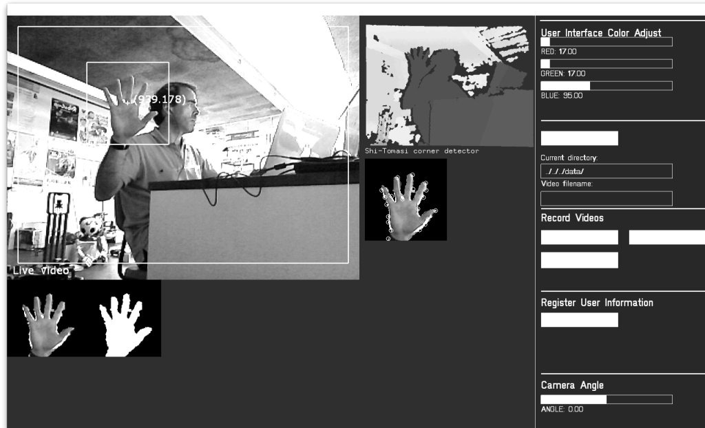
Figure 73. The Shi-Tomasi corner detector operator feature extraction
