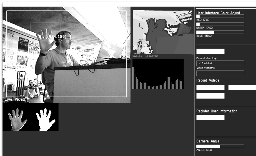
Figure 74. Radial Signature operator feature extraction.
