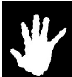
Figure 14. Hand blob extracted from the depth image and used for feature extraction.
