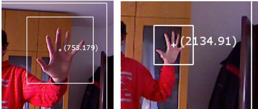
Figure 12. Bounding box size relative to the hand distance to the camera.
