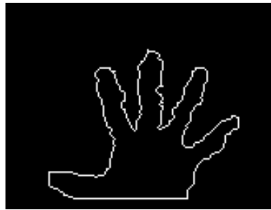
Figure 15. Hand contour extracted from hand blob.
