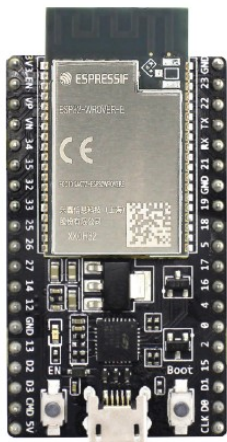
Figura 2.10: Microcontroller ESP32, ESPRESSIF 2023
