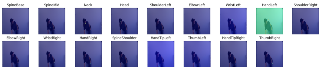
Figure 6.7: Inference results on a sample image from the Pandora dataset. The left hand is out of the image, which is noticed by the model's generated heatmaps for the keypoints of that region, which contain a different tone of blue background (low confidence).
