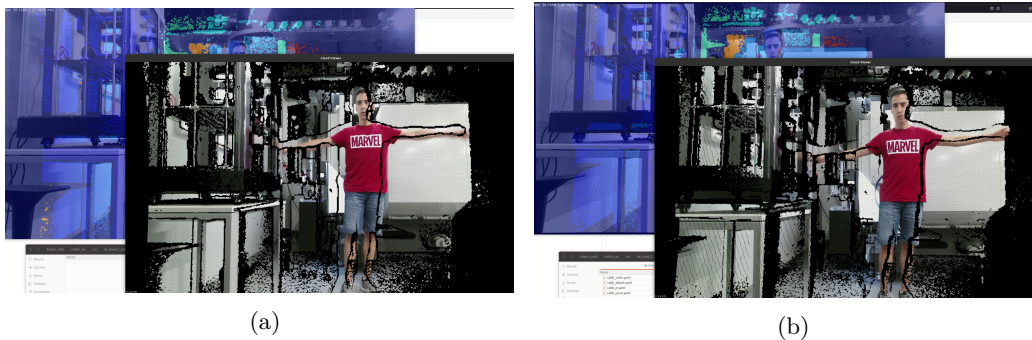
Figure 6.13: Visual comparison between: (a) default Kinect v2 calibration settings, and (b) manual calibration results.
