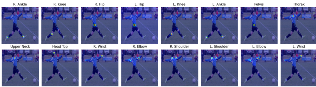
Figure 6.6: Inference results on a sample image from the COCO dataset. The position of the heatmap peaks is mostly correct, but can have problems distinguishing sides of the body.
