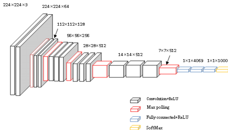
Figure 3.9: VGG neural network architecture [125].
