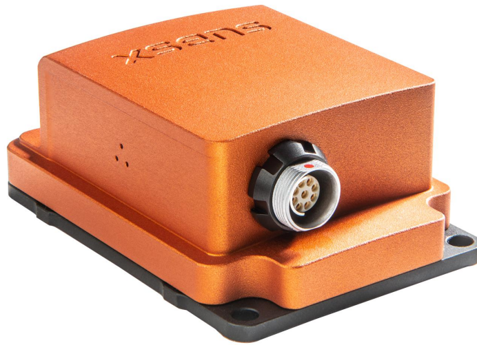
Figure 2.7: MTi-100, one of the IMU's part of the MTx line of sensors from Xsens [Farnell, 2023].
