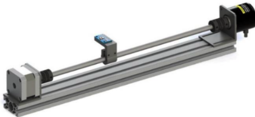
Figure 2.11: Motion sensor' testing apparatus, developed by L. Yavan and C. Tepe [Makalesi et al., 2021].
