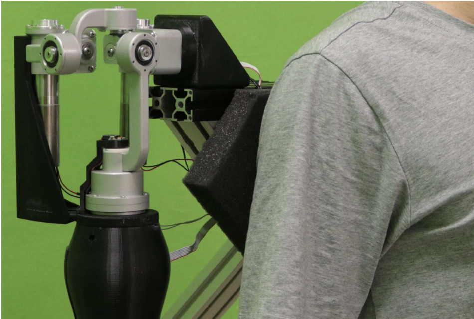
Figure 2.4: Spherical active joint developed by [Mghames et al., 2019].
