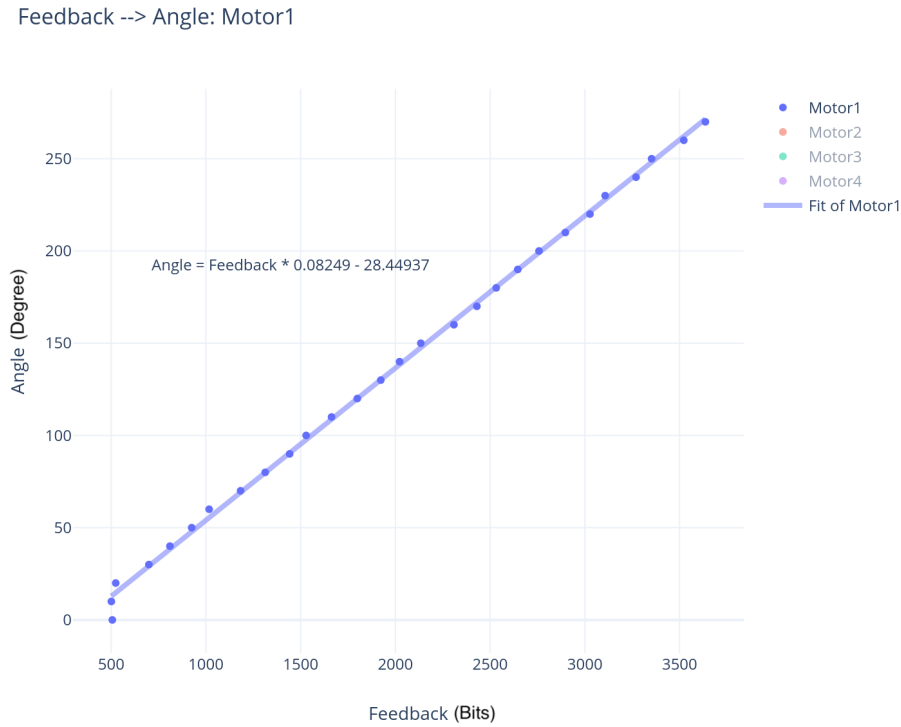
Figure 4.15: Graph that shows the relationship between feedback value and angle of the first servo motor.
