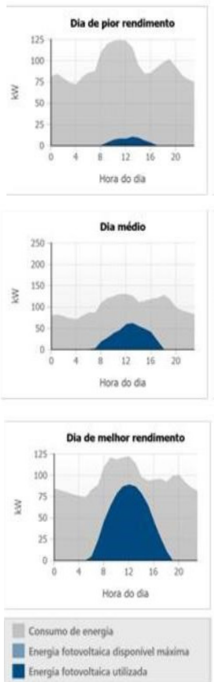
Figure 1. Estimates of PV energy produced (SMA Simulator)
