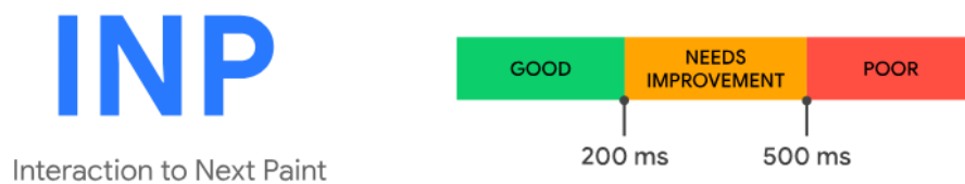
Figure 6 – A scale of the INP metric [46].
