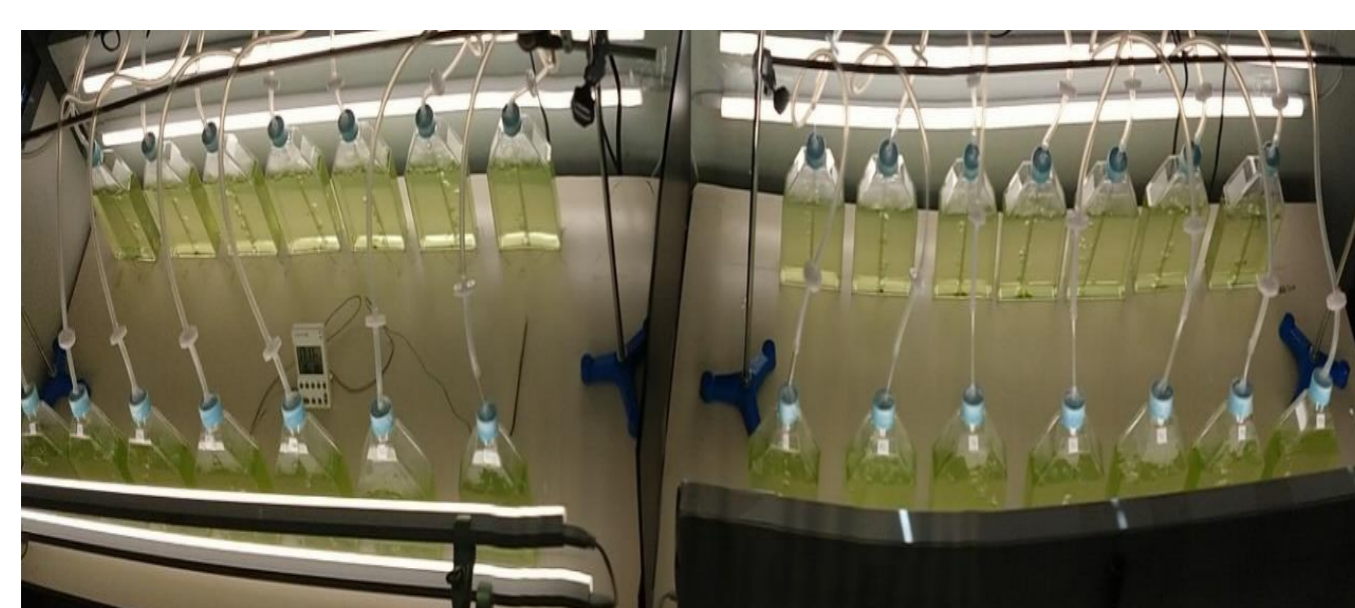
Figure 1. Microalgae cultivations based on full factorial experimental planning (2 n , n=4) with three central points.
