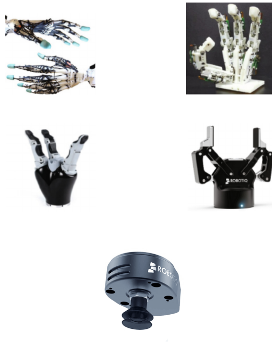
Figure 2.9: Robot End Effectors [8] (Left to Right): (Top) Human hand and 4 Finger hand, (Middle) 3 finger hand and Parallel gripper, (Bottom) Vacuum gripper
