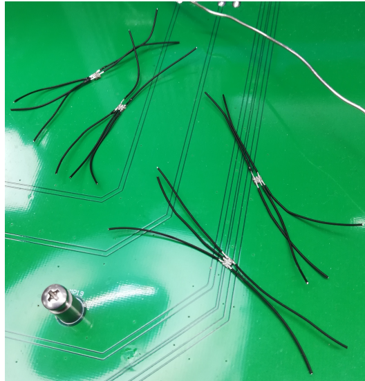
Figure 6.10: The new sensors being soldered
