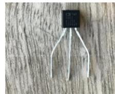
Figura 3 - Sensor LM35 e sensor TMP36
