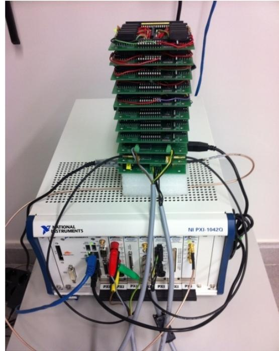
Figure 1. VISIR hardware platform at University of Deusto
